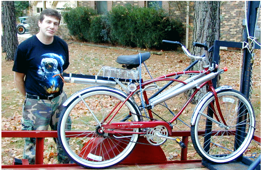
Glen May and Tim Picken's Hybrid Rocket-powered Bicycle
