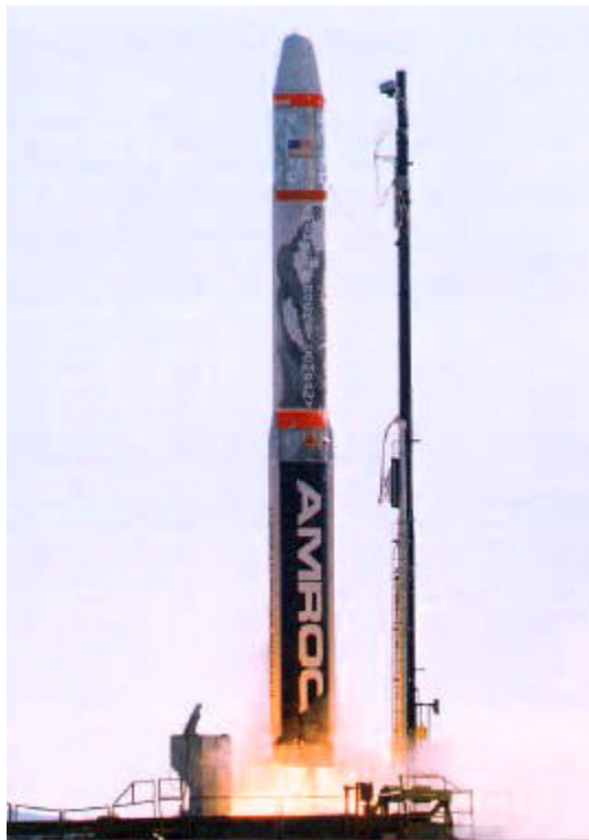
AMROC's first hybrid rocket failed to leave the launch pad when the LOX valve froze.
