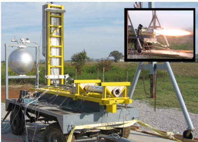
Project HALO Tube Launch – 1 Flight Motor Static Test #2.
